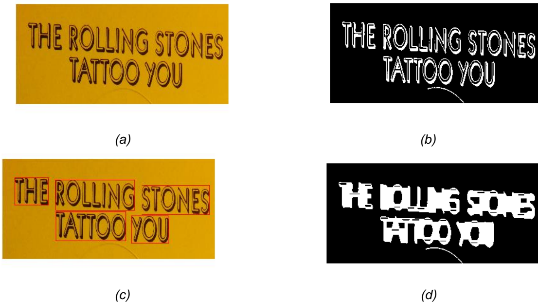
Figure 17 – Text Segmentation Example (a) Original image (b) Image after thresholding (c) Image after dilation (d) Contours from image
